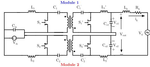
Fig. 1. Grid-connected gallium nitride (GaN) based DMCI with high-frequency (HF) transformer isolation.
