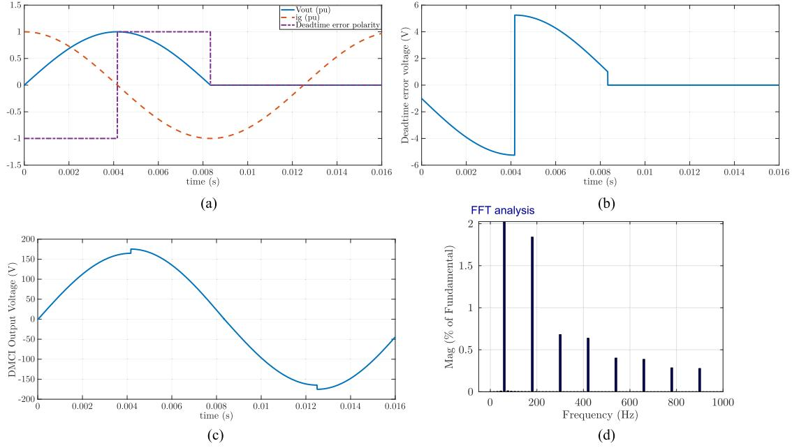
**Fig. 6.** (a) Module 1 output voltage, grid current, and deadtime error voltage polarity for ZPF (lead), (b) deadtime error voltage for module 1, (c) overall output voltage of the DMCI due to the deadtime, and (d) spectrum of the DMCI output voltage.
