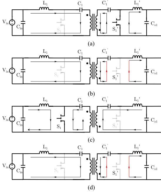
**Fig. 3.** Modes of operation of module 1 for ZPF case with  $i_g > 0$ . (a)  $S_1 = 0, S'_1 = 1$ . (b)  $S_1 = 0, S'_1 = 0$  (Deadtime). (c)  $S_1 = 1, S'_1 = 0$ . (d)  $S_1 = 0, S'_1 = 0$  (Deadtime).
