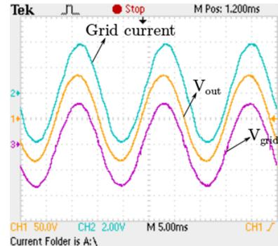
Fig. 18. Performance of the DMCI at higher grid current showing reducing harmonic distortion. Scale:  $V_{grid} = 50$  V/div,  $V_{out} = 50$  V/div, and  $i_{grid} = 2$  A/div.
