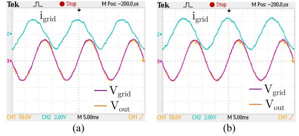
Fig. 12. Performance of the DMCI under ZPF using (a) deadtime and (b) proposed deadtime elimination approaches. Scale:  $V_{\text{grid}}$  and  $V_{\text{out}} = 50 \text{ V}/\text{div}$ ,  $i_{\text{grid}} = 2 \text{ A}/\text{div}$ .
