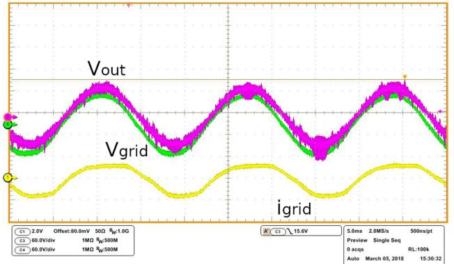
Fig. 17. Increased harmonic distortion in the grid current when there is a mismatch in the deadtime of the two modules of the DMCI. Channel 1: Grid current ( $i_{grid}$ : 2 A/div); channel 3: DMCI output voltage ( $V_{out}$ : 60 V/div); channel 4: grid voltage ( $V_{grid}$ : 60 V/div).
