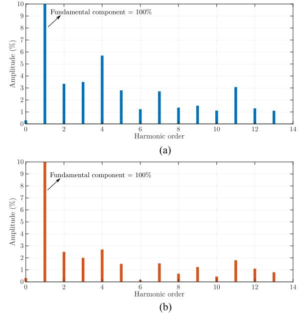
Fig. 13. Harmonic spectrum of the grid current for the ZPF operation (a) with conventional deadtime and (b) with proposed deadtime elimination approaches.
