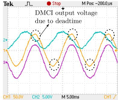
Fig. 14. DMCI output voltage in ZPF highlighted to show the jumps near the peak due to the deadtime effect. Scale:  $V_{grid}$  and  $V_{out} = 50$  V/div,  $i_{grid} = 5$  A/div.
