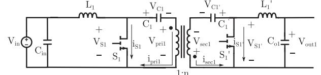
**Fig. 4.** Module 1 of the DMCI with various voltages and currents marked.
