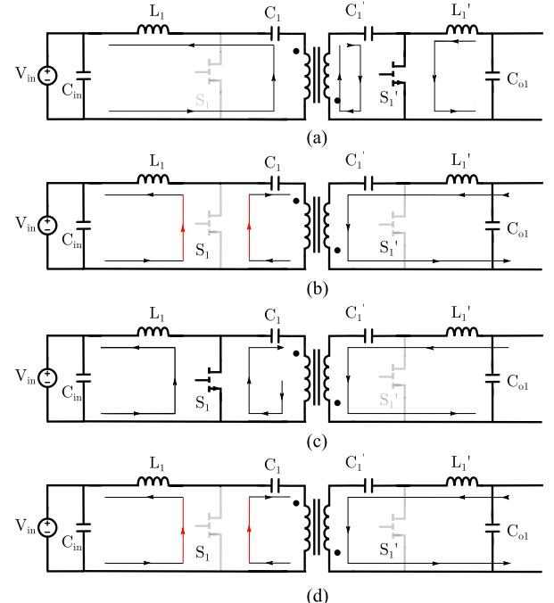
**Fig. 5.** Modes of operation of module 1 for ZPF case with  $i_g < 0$ . (a)  $S_1 = 0, S'_1 = 1$ . (b)  $S_1 = 0, S'_1 = 0$  (Deadtime). (c)  $S_1 = 1, S'_1 = 0$ . (d)  $S_1 = 0, S'_1 = 0$  (Deadtime).
