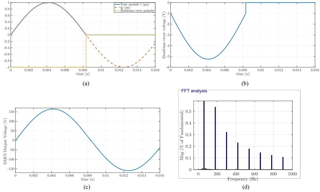
**Fig. 7.** (a) Module 1 output voltage, grid current, and deadtime error voltage polarity for UPF, (b) deadtime error voltage for module 1, (c) overall output voltage of the DMCI due to the deadtime, and (d) spectrum of the DMCI output voltage.
