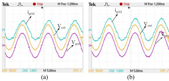
Fig. 15. Performance of the DMCI under UPF using (a) deadline and (b) proposed deadline elimination approaches. Scale:  $V_{grid}$  and  $V_{out} = 50$  V/div,  $i_{grid} = 2$  A/div.
