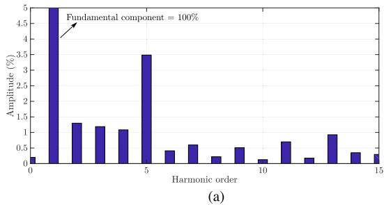
Fig. 16. Harmonic spectrum of the grid current for the UPF operation (a) with conventional deadtime and (b) with proposed deadtime elimination approaches.
