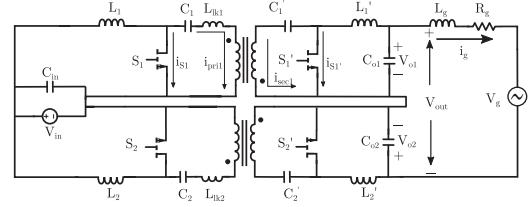
Fig. 8. Practical DMCI with the leakage inductance of the HF transformer.
