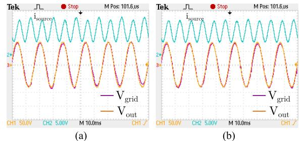
Fig. 19. Impact on the source current of the DMCI using (a) deadtime and (b) proposed deadtime elimination approaches. Scale:  $V_{grid}$  and  $V_{out} = 50$  V/div,  $i_{grid} = 5$  A/div.
