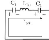
Fig. 9. HF transformer equivalent circuit during the overlap period.
