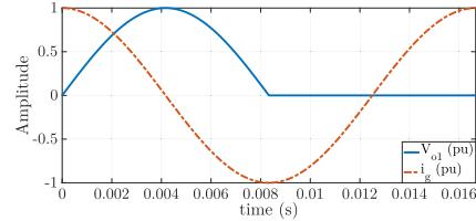
Fig. 2. Module 1 output voltage ( $v_{o1}$ ) and grid current ( $i_g$ ) for zero power factor (ZPF) (lead).
