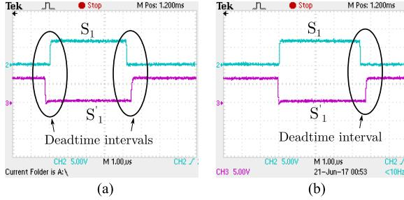
Fig. 11. Gate-drive pulses of  $S_1$  and  $S'_1$  when (a) the conventional deadtime approach is used, and (b) with the proposed deadtime elimination. Scale: Gating pulses = 5 V/div.
