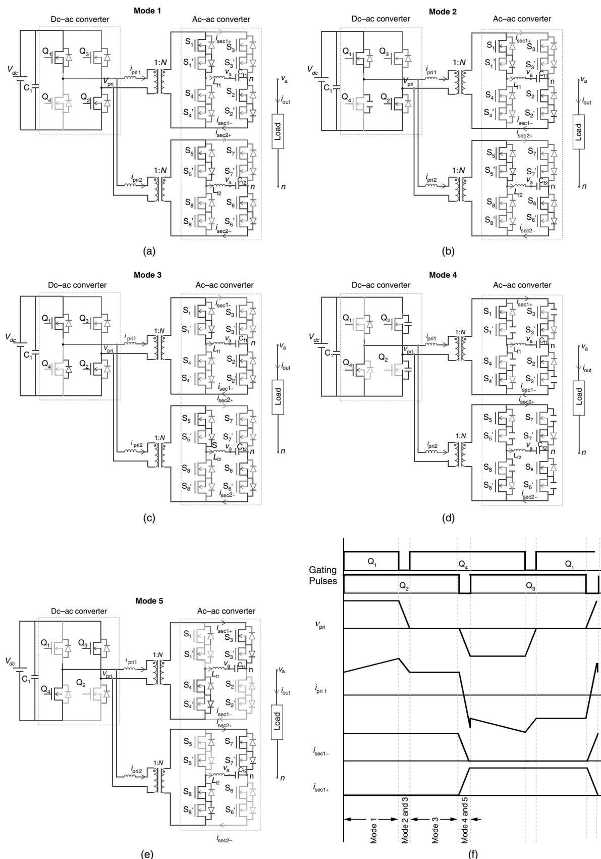
FIGURE 29.14 Modes of operation [1] for 120 V ac for input voltage in the range of 42–60 V ( $N = 4.3$ ): (a–e) topologies corresponding to the five operating modes of the overall dc–ac converter for positive primary current and for power flow from the input to the load. (f) Schematic waveforms show the operating modes of the HF inverter when primary currents are positive. The modes of operation of less than 42 V (i.e.,  $N = 6.5$ ) remain the same.
