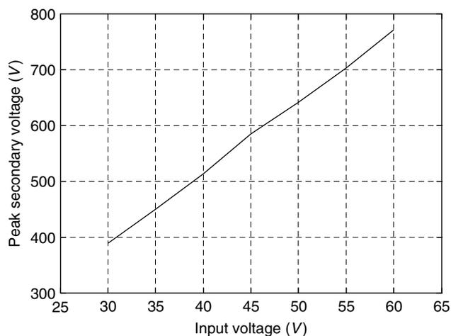
**FIGURE 29.21** Peak voltage across the ac–ac converter [1] with varying input voltage for a transformer primary leakage inductance of  $0.7 \mu\text{H}$ , output capacitance of  $240 \text{ pF}$  (for the devices of the ac–ac converter), and output filter inductance and capacitance of  $1 \text{ mH}$  and  $2.2 \mu\text{F}$ , respectively.
