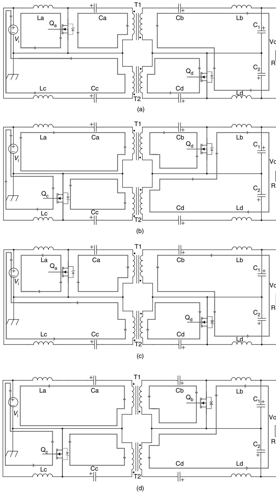
**FIGURE 29.3** Direction of the current flow [2]: (a) and (b) for positive load current and (c) and (d) for negative load current. (a) Mode 1, when  $Q_a, Q_d$  are ON and  $Q_b, Q_c$  are OFF; (b) Mode 2, when  $Q_a, Q_d$  are OFF and  $Q_b, Q_c$  are ON; and (c) and (d) are Modes 3 and 4 corresponding to negative load current.
