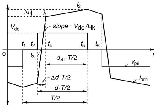
FIGURE 29.16 Transformer primary-side voltage and current waveforms [1].
