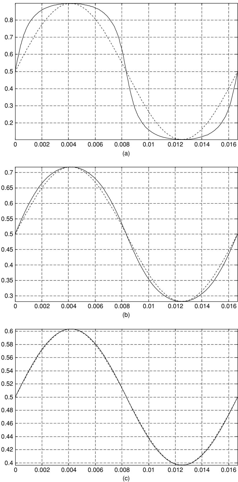
**FIGURE 29.5** The plotted waveforms [2] of  $D = (A + B)/C$  for variable transformer turns ratio (solid). (a)  $N = 2:1$ ; (b)  $N = 1:2$ ; and (c)  $N = 1:5$ , as compared with a standard sine wave (dash).
