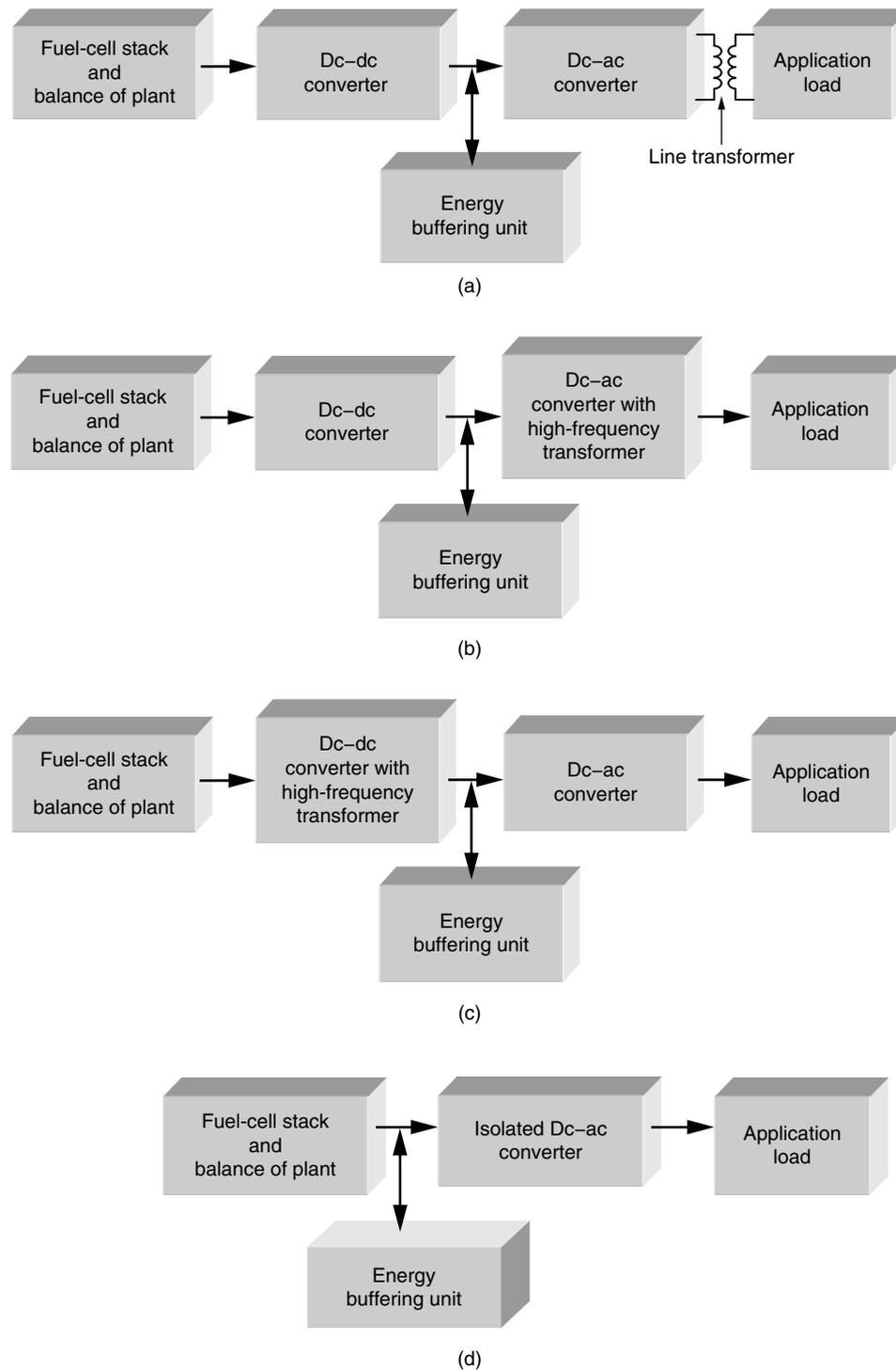
**FIGURE 29.1** Inverter power-conditioning schemes [1] with (a) line-frequency transformer; (b) HF transformer in the dc-ac stage; (c) HF transformer in the dc-dc stage; and (d) single-stage isolated dc-ac converter.
