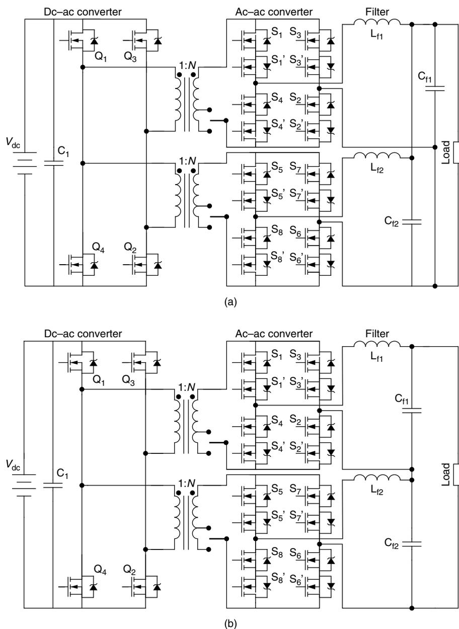
**FIGURE 29.12** Circuit diagrams [1] of the proposed fuel-cell inverter for (a) 120 V/60 Hz ac outputs and (b) 240 V/50 Hz ac outputs. A single-pole-double-throw (SPDT) switch enables adaptive tapping of the transformer.
