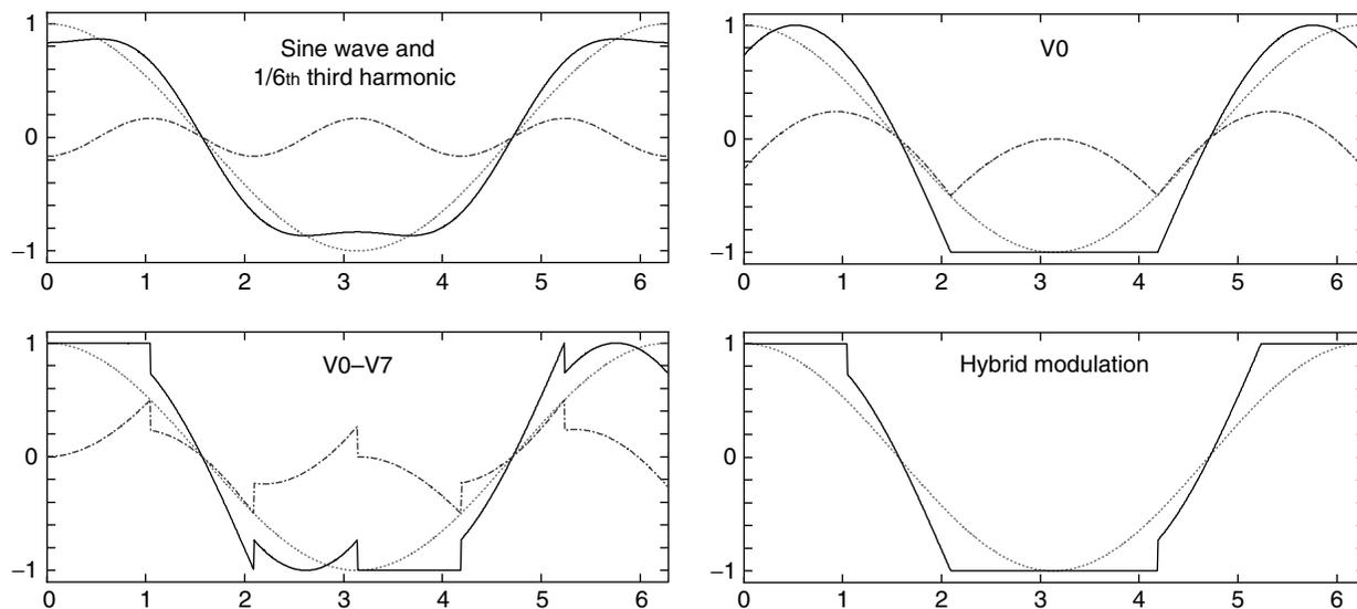
**FIGURE 29.26** Modulation functions corresponding to sine wave (with 1/6th third harmonic),  $V_0$ ,  $V_0$ - $V_7$  SVMs, and HM schemes. Blue and red traces represent zero sequence and sinusoidal signals. Black trace is the modulating signal.
