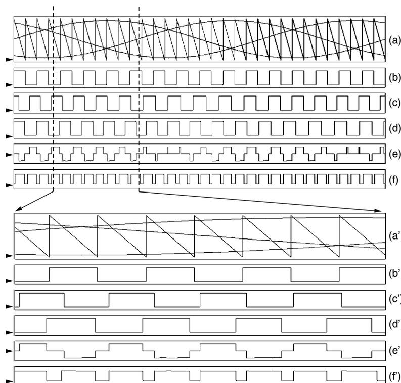
**FIGURE 29.24** Key waveforms [13] of the primary-side dc-ac converter in one cycle and enlarged view of the interval between two dot lines; (a) three-phase sine-wave references and carrier signal; (b) Q: square wave with half frequency of the carrier; (c) UT: gate signal for the upper switch of phase U; (d) VT: gate signal for the upper switch of phase V; (e)  $V_{uv}$ : output of phase U and V; and (f)  $V_{rec}$ : output waveform of the rectifier.
