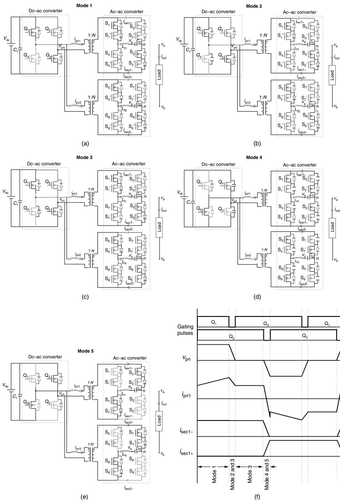
FIGURE 29.15 Modes of operation [1] for 240 V/50 Hz ac output for an input-voltage range of 42–60 V (corresponding to  $N = 4.3$ ): (a–e) topologies corresponding to the five operating modes of the inverter for positive primary and positive filter-inductor currents. (f) Schematic waveforms show the operating modes of the dc-ac converter when primary currents are positive. The modes of operation of less than 42 V (corresponding to  $N = 6.5$ ) remain the same.
