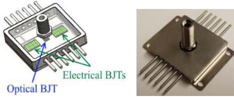
Fig. 3. Fabricated Darlington OTPT in one package.
