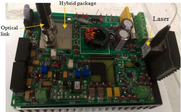
Fig. 23: Fabricated board, which includes power circuit, control circuit, laser, and laser driver [8], [9].
