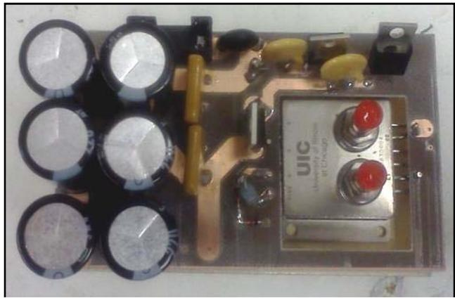
**Fig. 18:** Boost converter prototype showing OTPT-based optically-triggered packaged hybrid power device [7].
