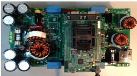
Fig. 15. Experimental prototype of the DMCI. It shows the TMS320F28335 DSP-based digital controller on the top feeding the DMCI power stage at the bottom.
