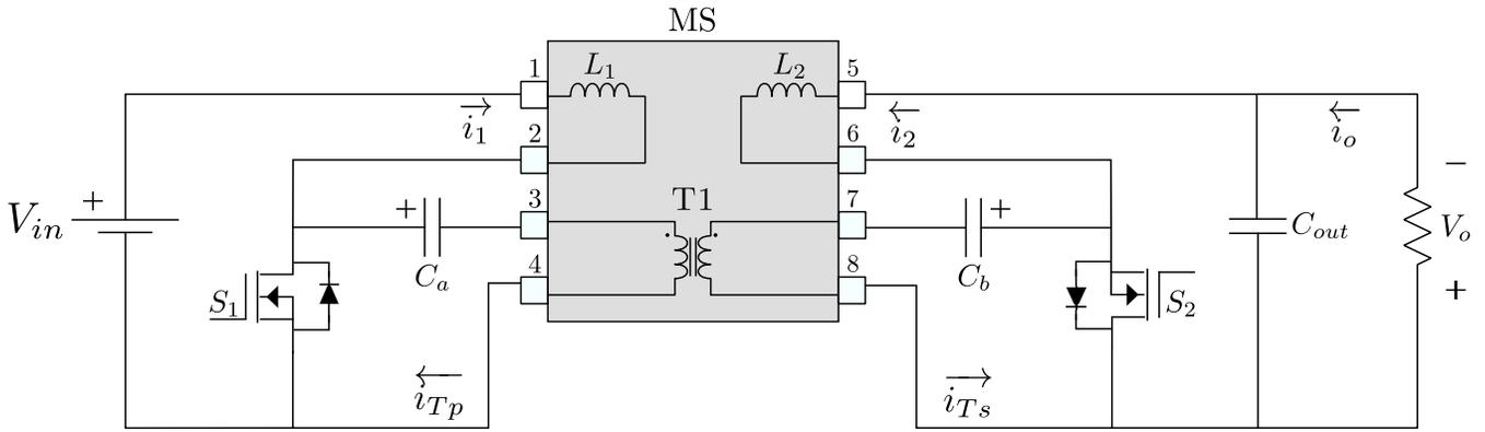
Fig. 1: Basic isolated Ćuk converter topology.
