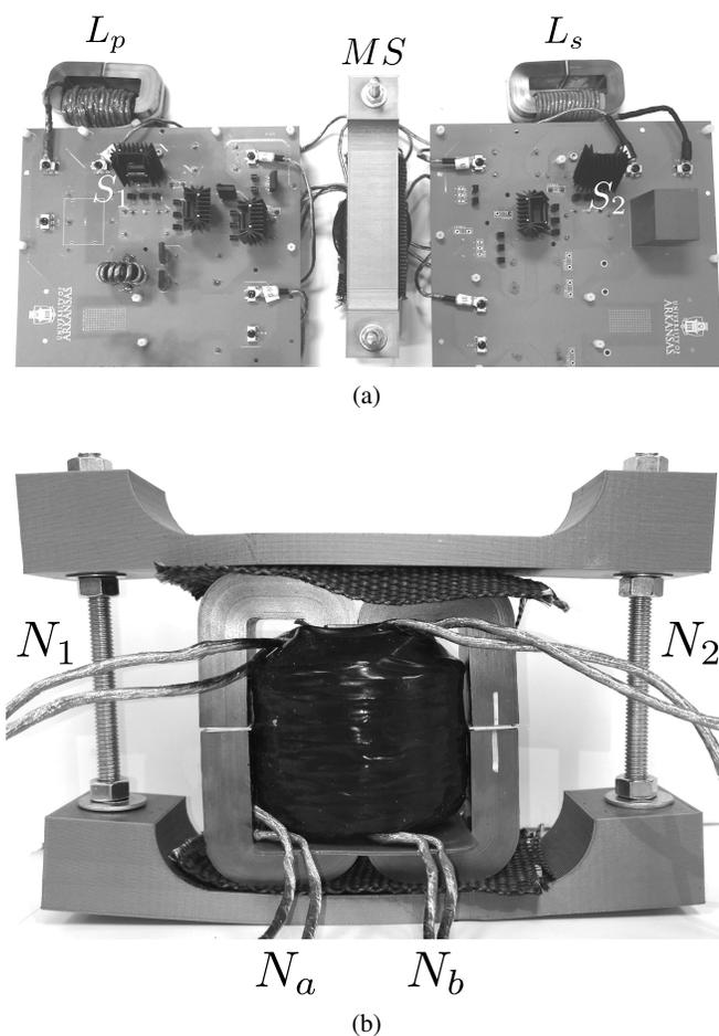
Fig. 7: Experimental setup: (a) Ćuk converter prototype (b) Proposed MS.
