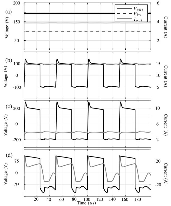
Fig. 6: Simulation results for the proposed IM with a 2 to 1 ratio: (a)  $V_{out}$  and  $i_{out}$ . (b)  $V_{Ls}$  and  $i_1$ . (c)  $V_{Ls}$  and  $i_2$ . (d)  $V_{T1}$  and  $i_{T1}$ .
