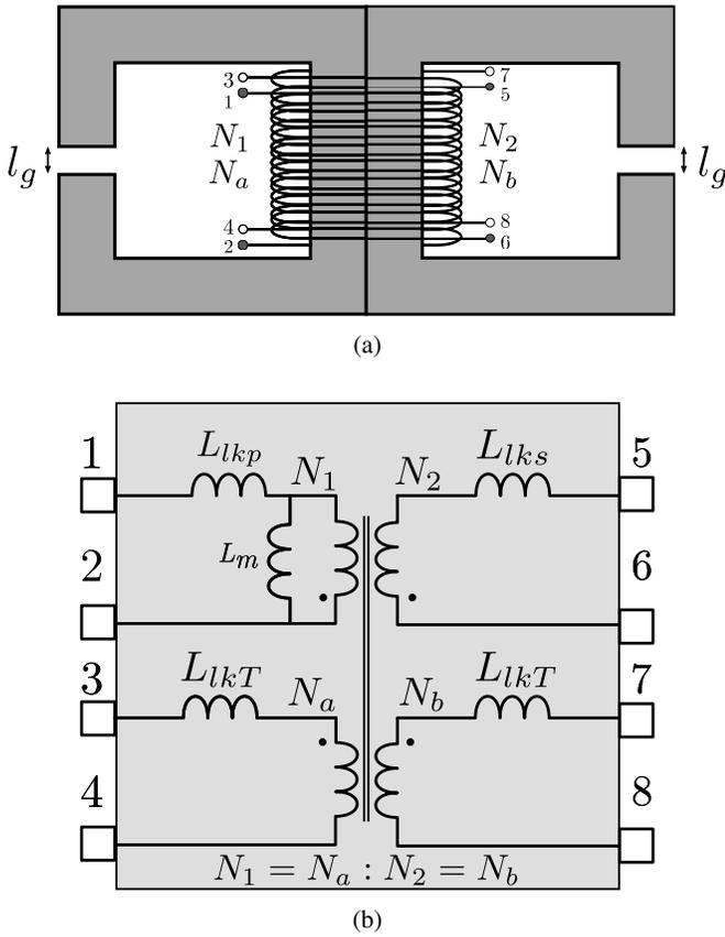
Fig. 3: Proposed IM: (a) MS. (b) Equivalent circuit.
