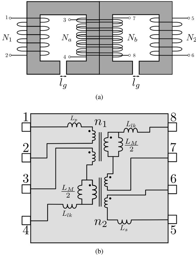
Fig. 2: Ćuk IM [11]: (a) MS. (b) Equivalent circuit.
