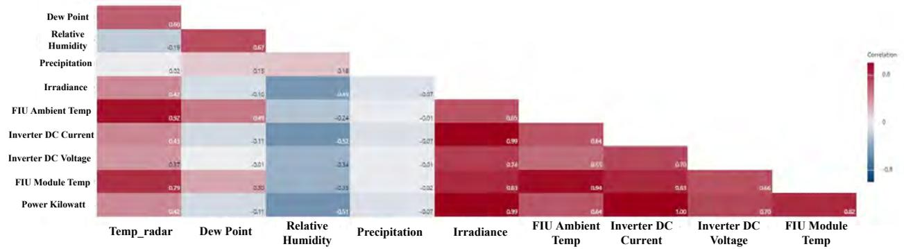
Fig. 8. Correlation study of inverter DC input with weather data
