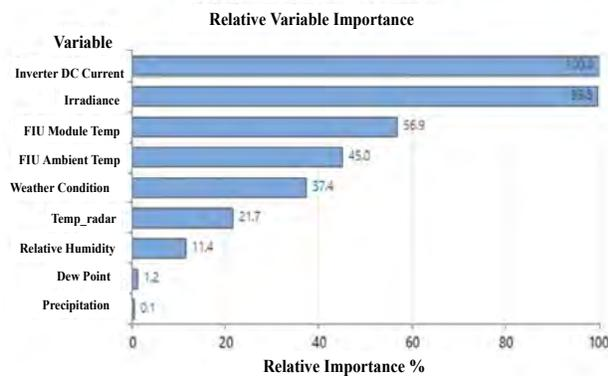
Fig. 9. Top five features in predicting inverter DC voltage
