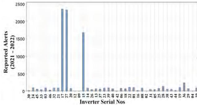
Fig. 7. Fault reporting inverters with fault counts (Dec, 2021 to Mar 2022)
