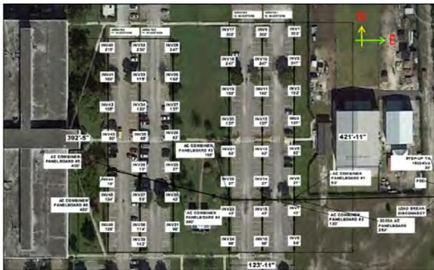
Fig. 1. Location of 46 grid-following solar inverter units
