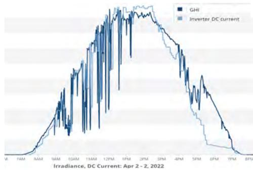
Fig. 10. Inverter DC input current with Irradiance profile over 24 hr.
