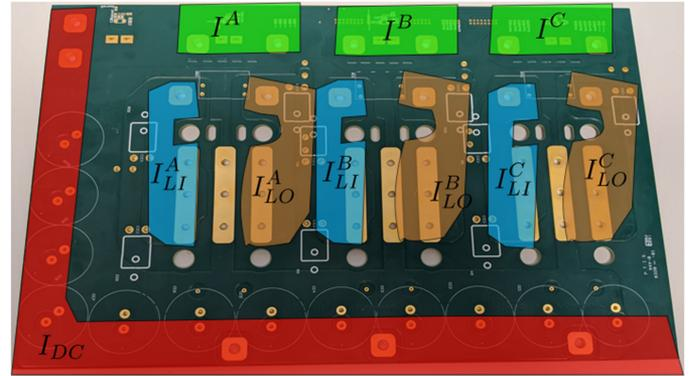
Fig. 8. Current patches in the high-power PCB for the major current carrying sections.
