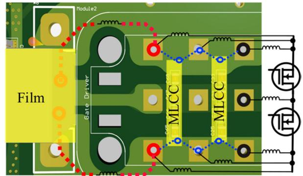
Fig. 20. High-frequency commutation loop layout of the blocking capacitors and the HB module.
