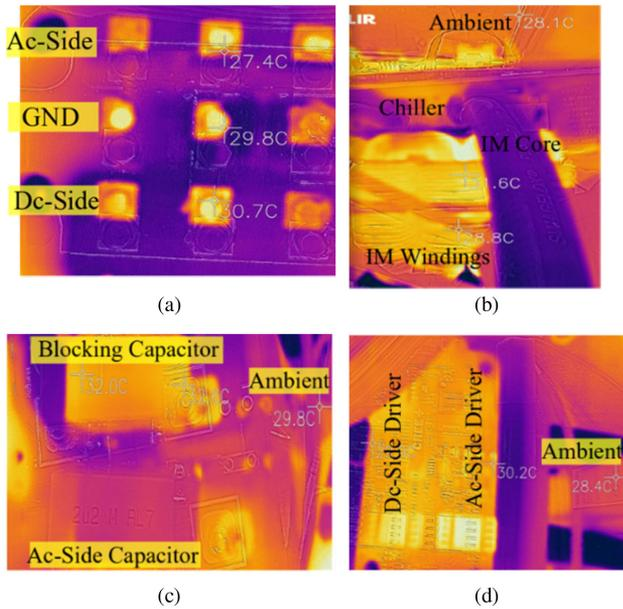
Fig. 22. Infrared image of the thermal performance of the UBS components. (a) HB SiC module. (b) Integrated magnetics core and windings. (c) Blocking capacitor as well as ac-side capacitor. (d) Cree's HB gate driver.
