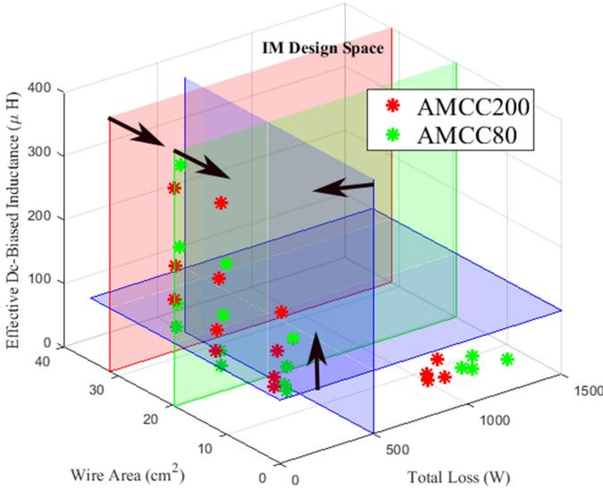
Fig. 12. Magnetics design space with imposed limits on losses, window is of the core (red plane for AMCC200 and green plane for AMCC80), and minimum inductance required.
