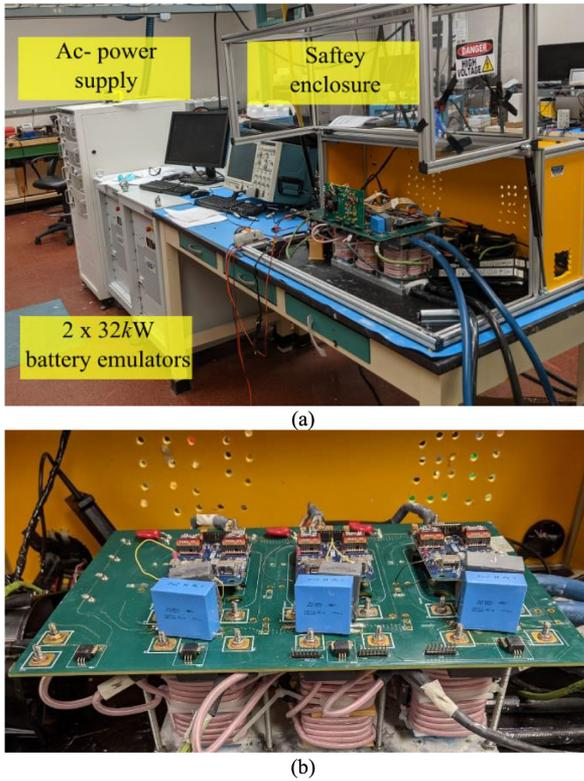
Fig. 24. (a) IM-DMCR experimental setup. (b) Power-stage components and board of the IM-DMCR.
