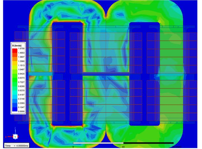
Fig. 14. Flux density field distribution on the IM-DMCR at the peak high-frequency current ripple and peak low-frequency bias for ac- and dc-side windings.
