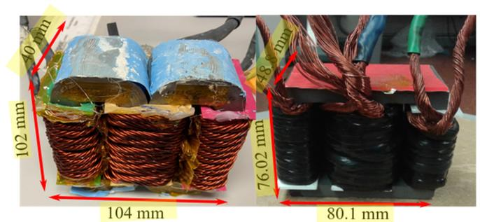
Fig. 10. Side by side comparison of iron powder and Metglas-material-based IM with relatively the same size.
