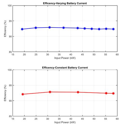
Fig. 26. Efficiency of the experimental DMCR for two different battery modes with varying power.
