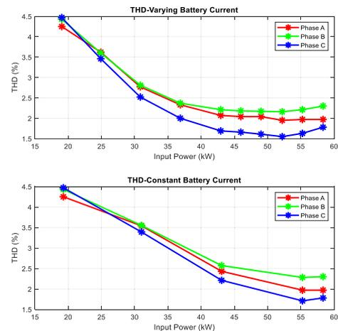
Fig. 27. THD in the experimental setup at two different battery modes with varying power.
