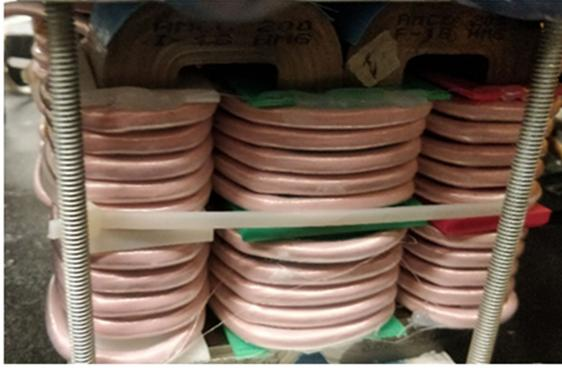
Fig. 15. Fabricated IM comprising Litz wire and Metglas cores.
