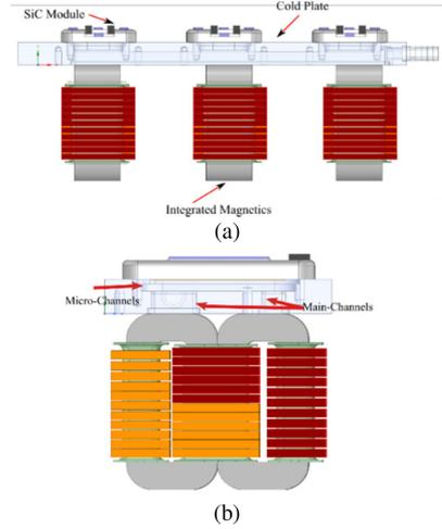
Fig. 21. Cooling solution for the high-power IM-DMCR. (a) Side view (b) front view.
