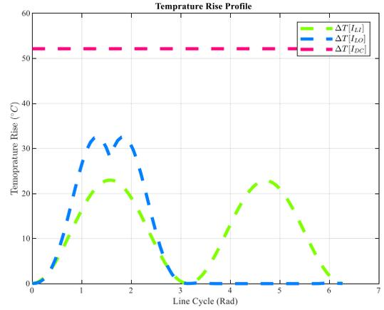
Fig. 7. Temperature rises in the ac side, dc side of the IM, and dc current in the sample copper sample.
