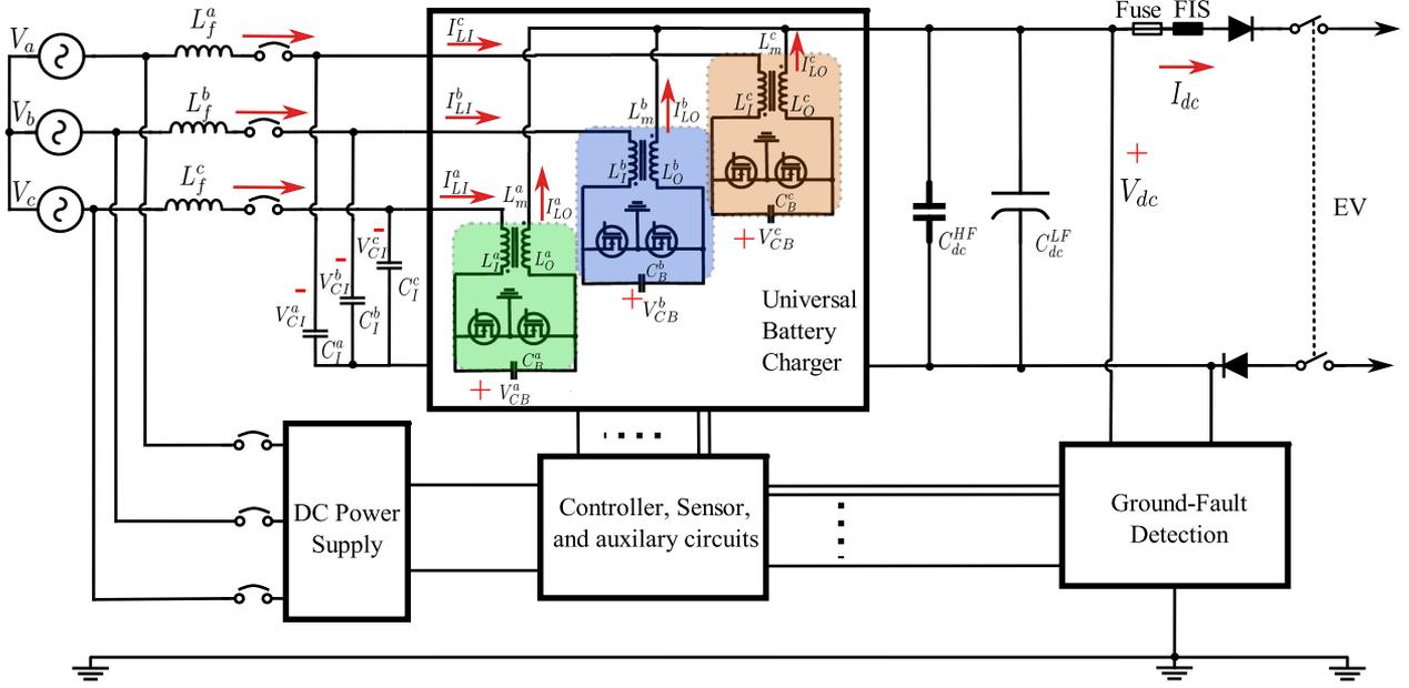
Fig. 1. Three-phase IM-DMCR topology in a UBS.
