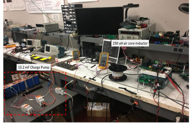
Fig. 17. DP test setup for characterization of the 1700 V SiC module.
