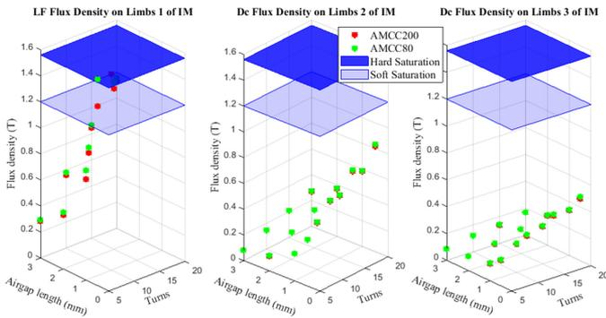
Fig. 13. Maximum flux density at peak current for both ac-side and dc-side windings in the integrated magnetics.
