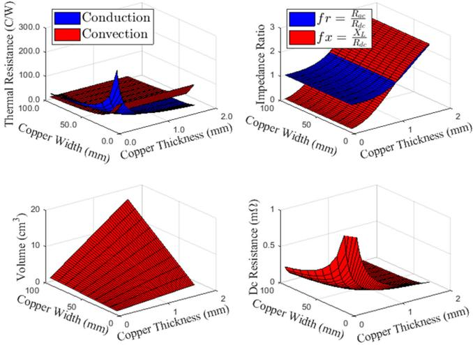
Fig. 5. Sweeping design variables with copper width and thickness.
