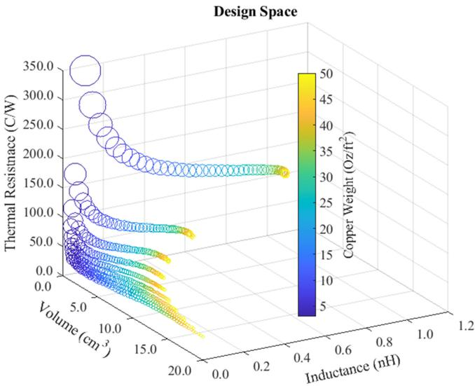
Fig. 6. Five-dimensional design space for the HC-PCB.
