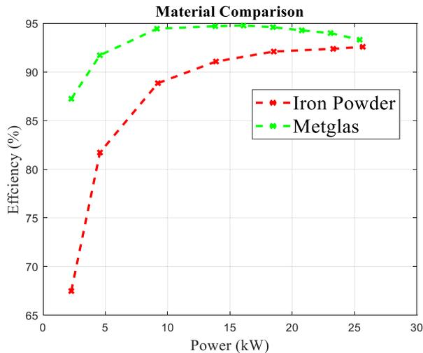
Fig. 9. Comparison of efficiencies of two IMs (for one IM-DMCR module) developed using iron-powder and Metglas materials.
