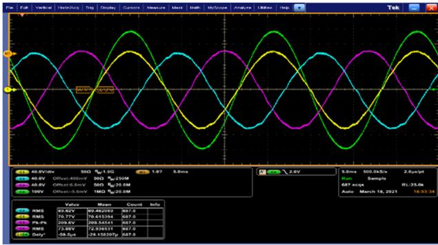
Fig. 28. Steady-state time-domain results of the three-phase input current and phase A input voltage. The yellow curve is phase A current (40 A/div), the blue curve is phase B current (40 A/div), the purple curve is phase C current (40 A/div), and the green curve is phase A voltage (100 V/div).
