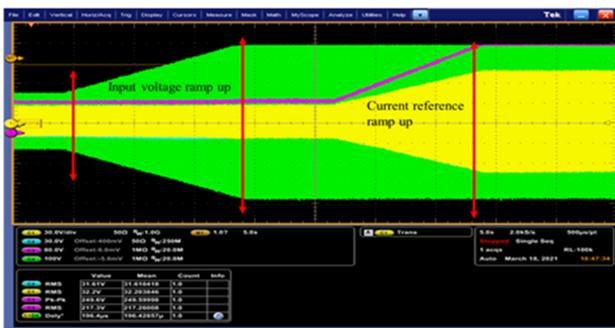
Fig. 29. Sequence of increasing the power on the UBS setup from 20% of the rated power to the rated power.
