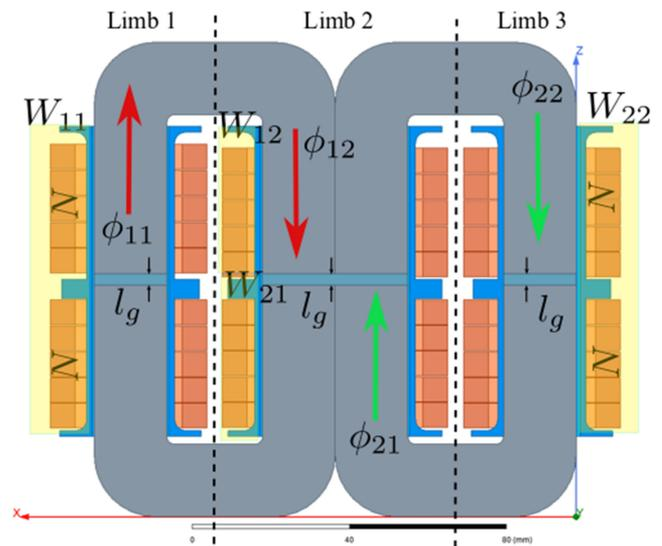
Fig. 11. IM design architecture for high-power IM-DMCR with double C cores.
