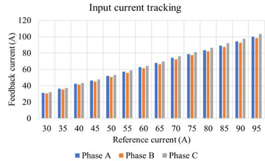
Fig. 25. Input current feedback and reference for phases A, B, and C.
