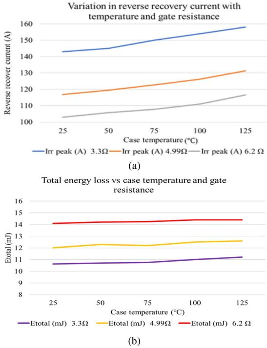
Fig. 18. (a) Reverse recovery current profile. (b) Total switching energy loss during turn-ON and turn-OFF transitions with case temperature and gate resistances.
