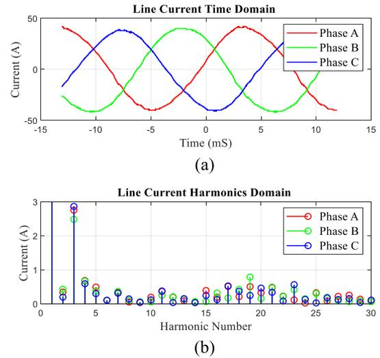
Fig. 23. (a) Three-phase line currents. (b) Spectral decomposition of the line current.
