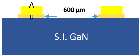
Cross-Section Diagram of GaN PCSS
