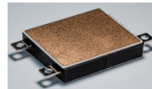
3D Integrated Double-Side-cooled GaN module from Univ. Arkansas (A. Emon)
