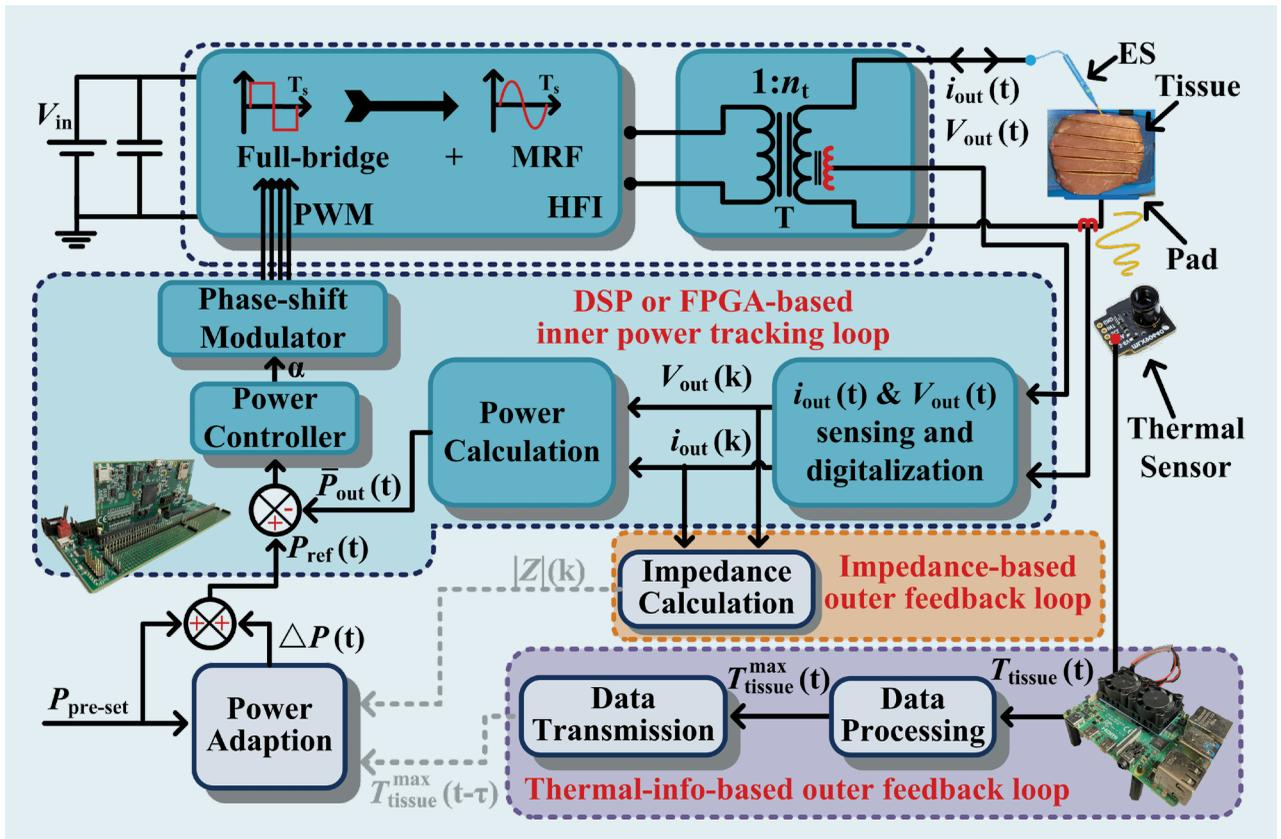
**FIG 4** Illustration of temperature- and tissue impedance-based outer feedback loop that autonomously modifies the setpoint of the inner power tracking loop.
