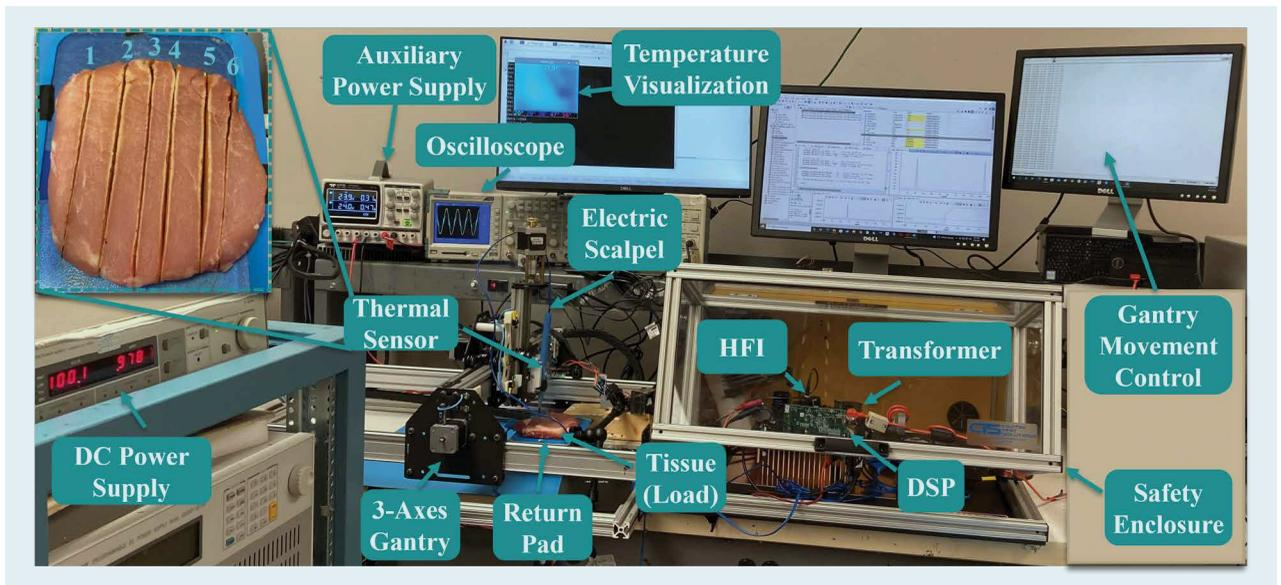
**FIG 5** A HFI-based experimental test bed setup for electro-surgery. Trace 3 in the upper left picture illustrates how precision power yields reduced collateral damage.
