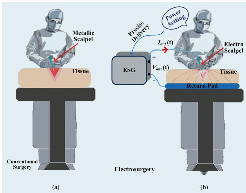
**FIG 2** Illustration of (a) conventional surgery using metallic scalpel and (b) power-electronics-based electrosurgery generator using an electroscalpel.
