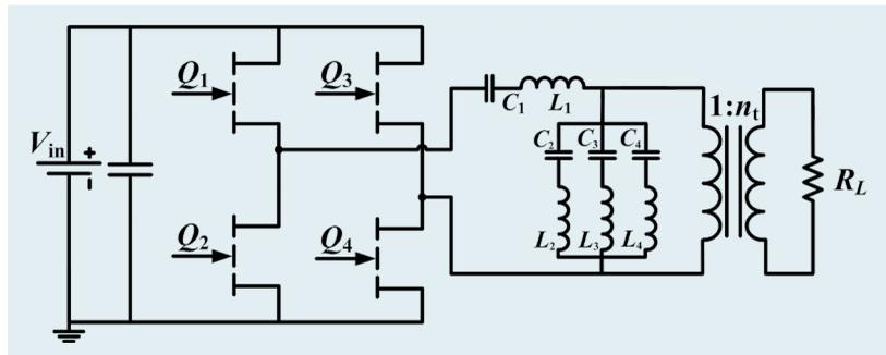
**FIG 3** The topology of the full-bridge and MRF based ESG. The biomedical load is represented by  $R_L$  whereas  $V_{in}$ ,  $Q_1$ - $Q_4$ ,  $C_1$ - $C_4$ , and  $L_1$ - $L_4$  represent dc input, GaN devices, resonant capacitors, and inductors, respectively. The transformer for galvanic isolation and voltage boost-up with a turn ratio of  $n_1$  is articulated as well.
