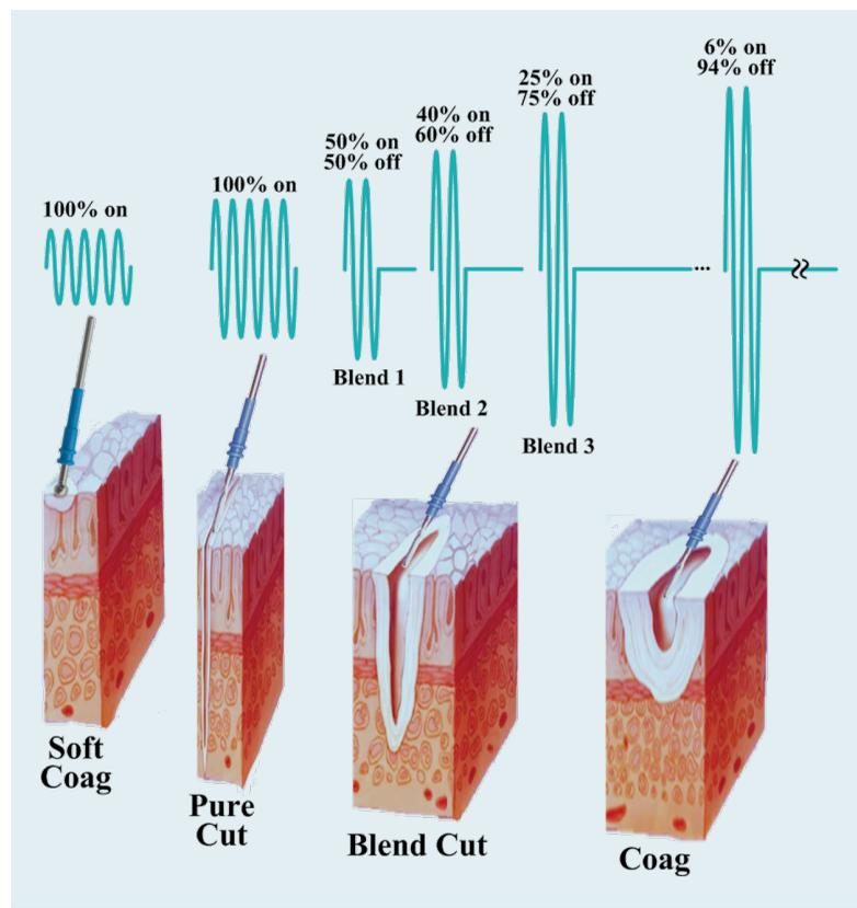
**FIG 1** Illustration of some electrosurgery modes capturing electrical waveforms for cutting, blending, and coagulation and their physical manifestations.
