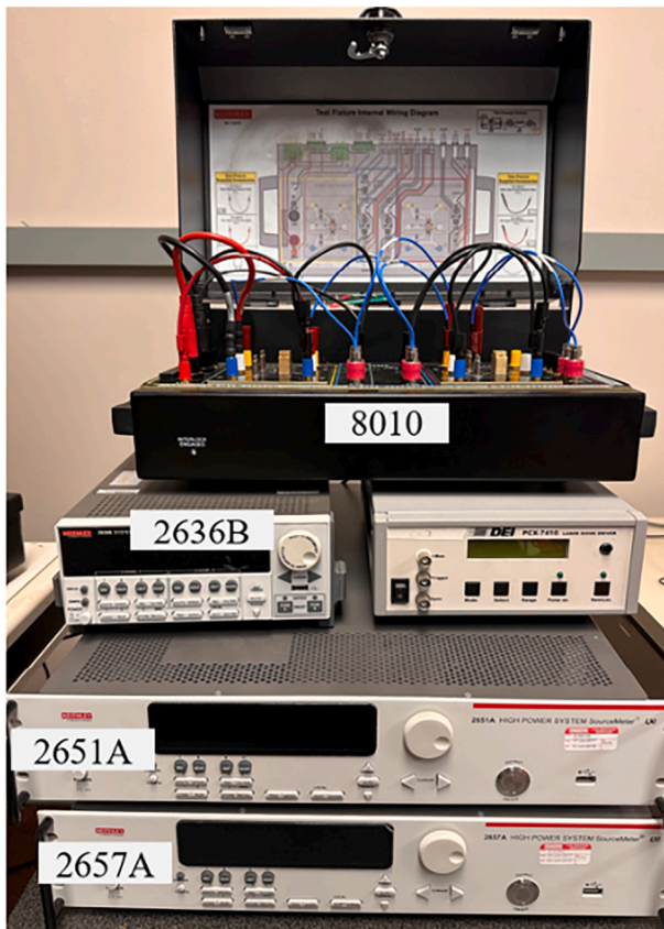
Fig. 6. Keithley instruments to characterize DUTs.
